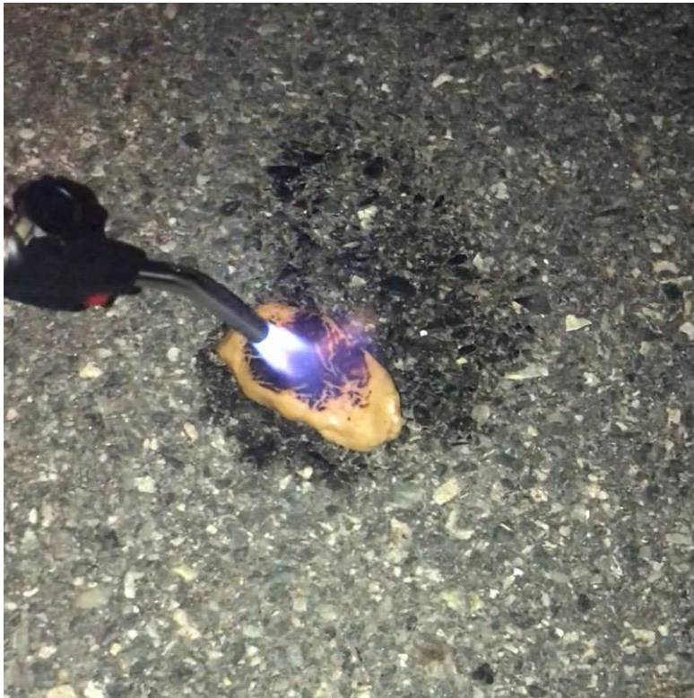
Figure A.5: Sample being burned with propane torch outside of Thayer. The torch scorched the top of the sample but never caught on fire.
