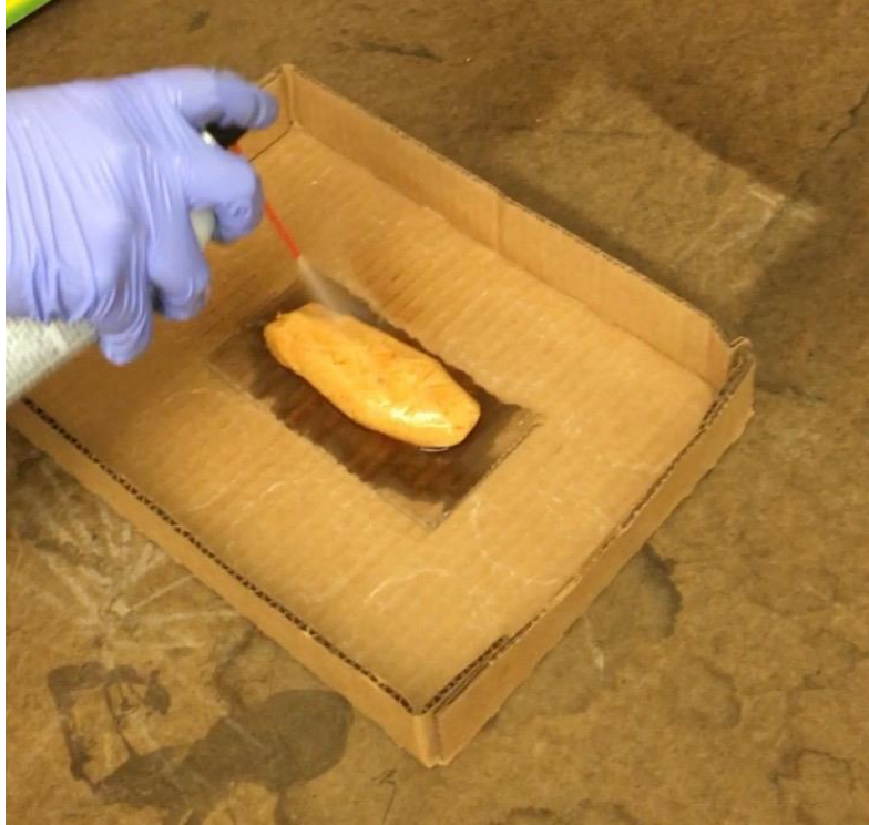
Figure A.4: Testing freeze spray to solidify sample. Sample was chilled but did not freeze and spray left a liquid residue.
