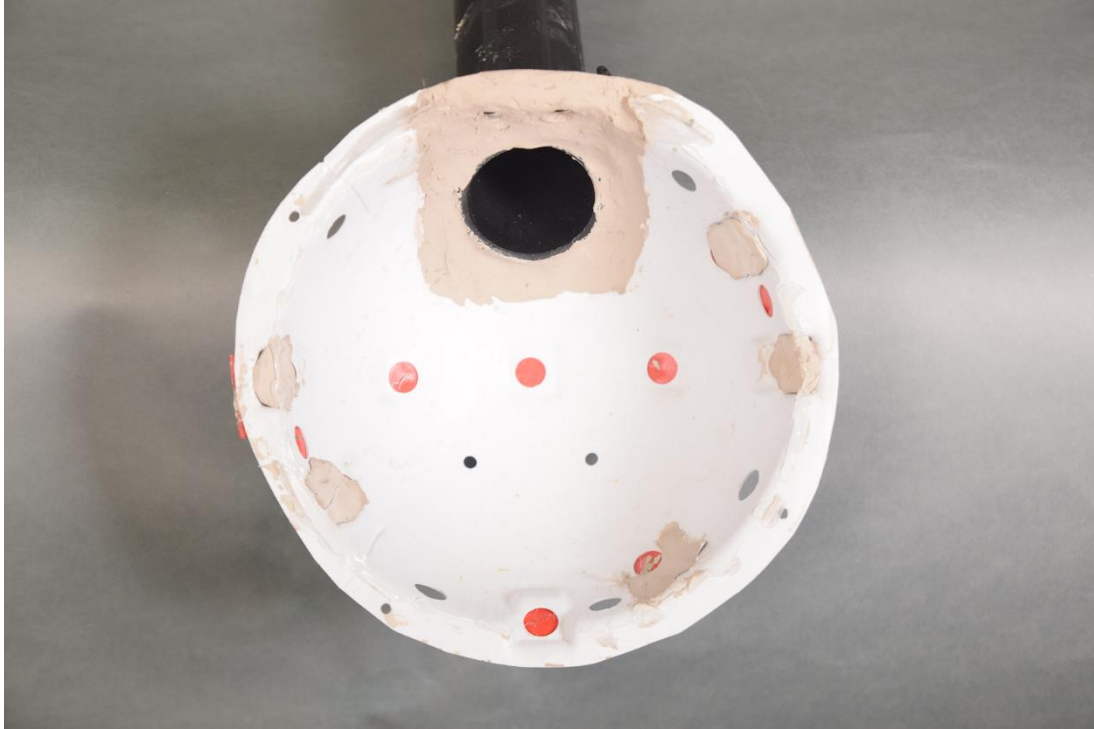
Figure F.7: Prototype 5 filled with molding clay to test the effect jet and vacuum mounting faces had on airflow and suction.
