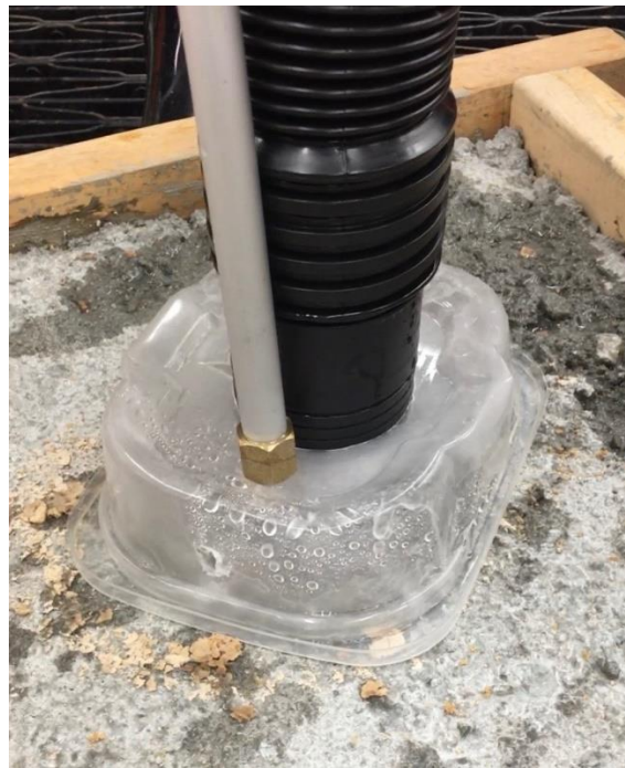
Figure C.1: Prototype 0 - Proof of concept prototype developed for PDR presentation, using tupperware and hose-attached pressure washer.
