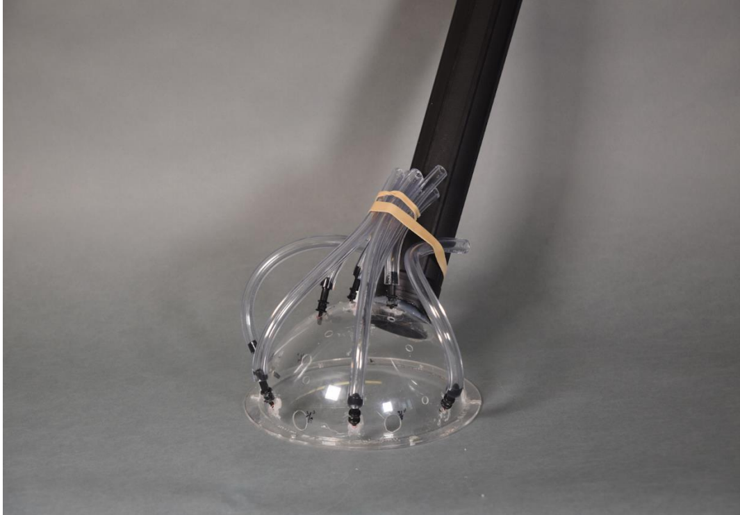
Figure C.5: Prototype 3: 7 in dome utilizing 8 tubes(not 9 as shown below due to lack of necessary splitter at time of creation) This was the prototype demonstrated at the CDR presentation. 9 jets were added after the presentation.
