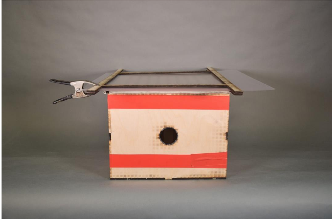
Figure F.8: Homemade thermoforming machine -- this machine was used for the creation of multiple iterations of prototype 5. It utilizes a 150CFM vacuum pulling air through a 16"x16" box. Custom clamps were made to hold and heat plastic using existing heating element.
