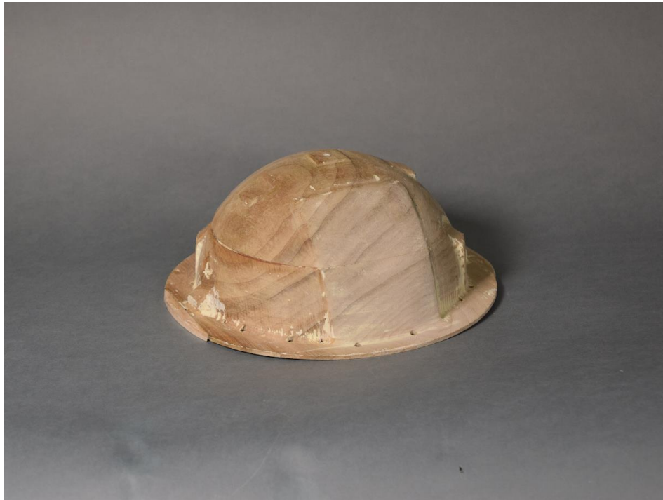
Figure F.5: Shopbotted wooden dome used as mold for domes in prototypes 5 & 6.
