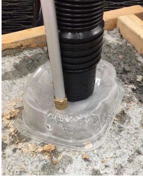
Figure A.6: Using pressure washer attachment in conjunction with vacuum to remove samples from test setup. The combination was able to remove both wet and dry samples.
