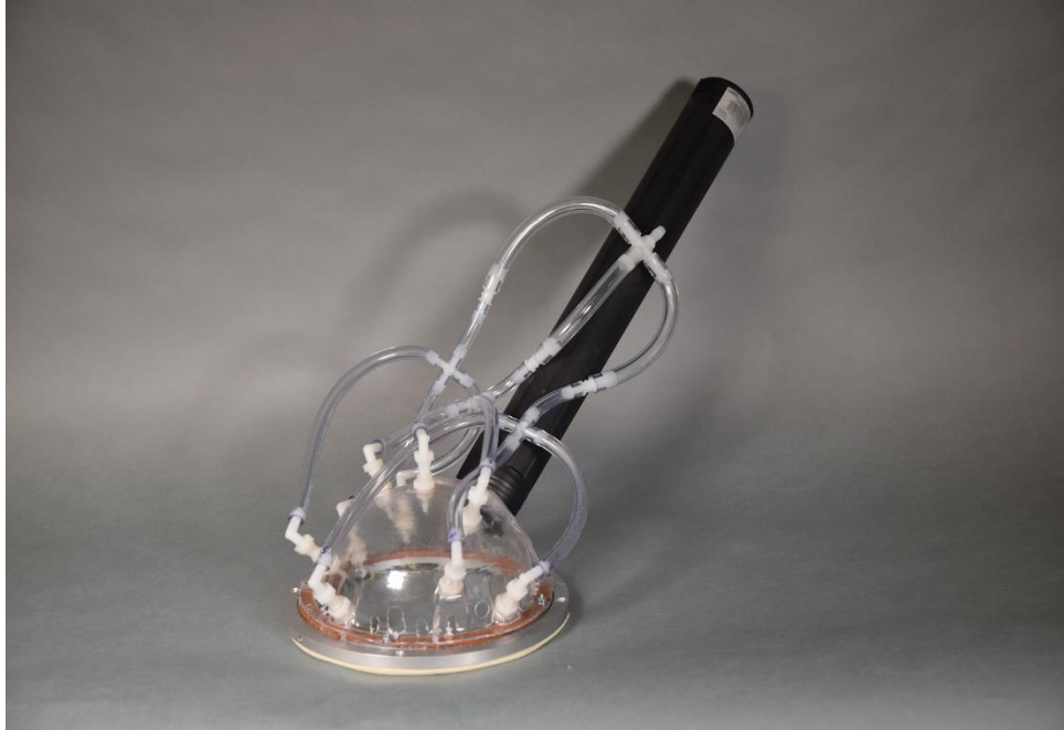
Figure C.8: Prototype 5 - 7in thermoformed dome, 9 jets utilizing 90 degree angle dome attachments. Note addition of gasket between dome and bearing to create reliable seal. This dome failed to develop desired suction due to turbulence developed by jet mounting faces.
