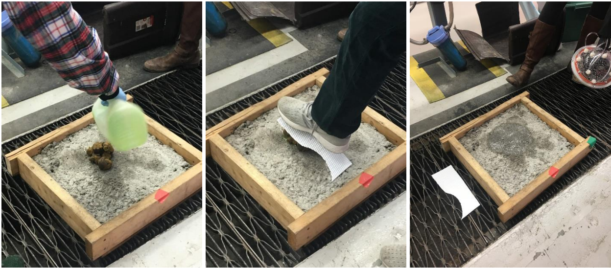
Figure G.3: Dog poop testing. Left: feces and liquid soap. Middle: stepping on the feces simulates a real-life worst-case scenario. Right: after the dome has been run.
