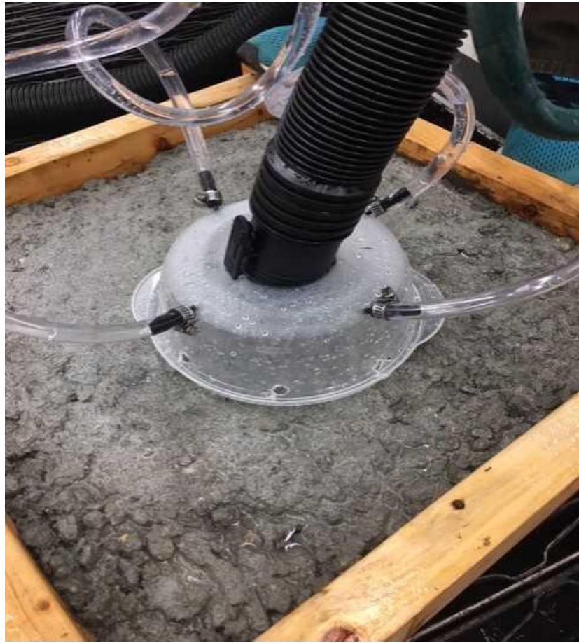
Figure C.2: Prototype 1 - Using pressurized jets and circular dome with vertically mounted vacuum to remove samples from test setup. The combination was able to remove both wet and dry samples.
