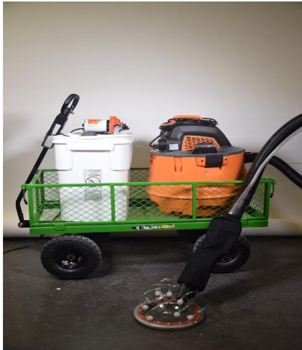
Figure 5: Fully assembled functional system (vacuum, tank, pump, cart head).
