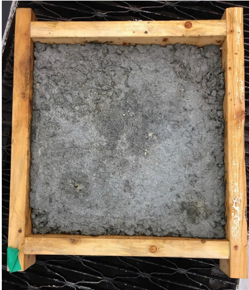
Figure A.1: 1.5'x1.5' test setup made out of 2x4s, plywood, and extra strength concrete. Surface has varied smoothness to replicate varying conditions found on city sidewalk.
