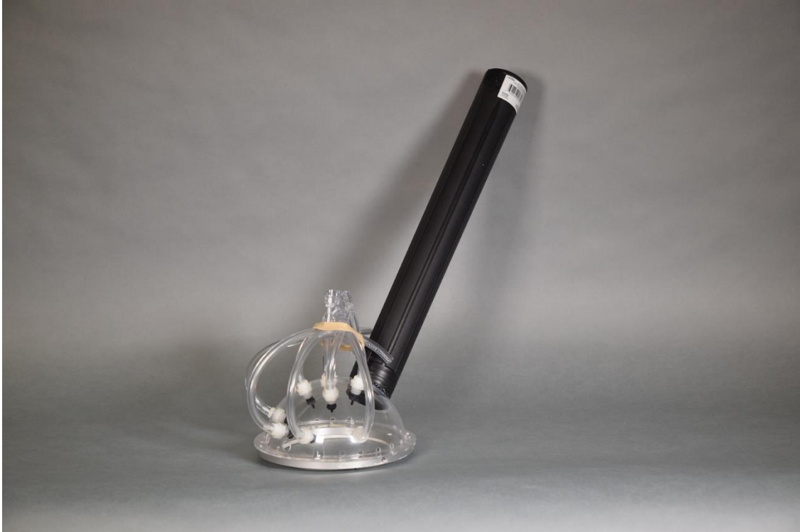
Figure C.7: Prototype 4 - 7in dome with 9 jets. Major addition from prototype 3 is the swivel bearing.
