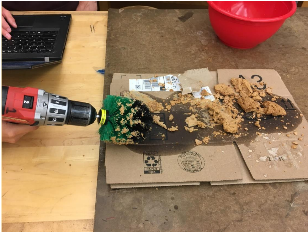
Figure A.3: Testing removal of wet sample using cylindrical brush attached to drill.
