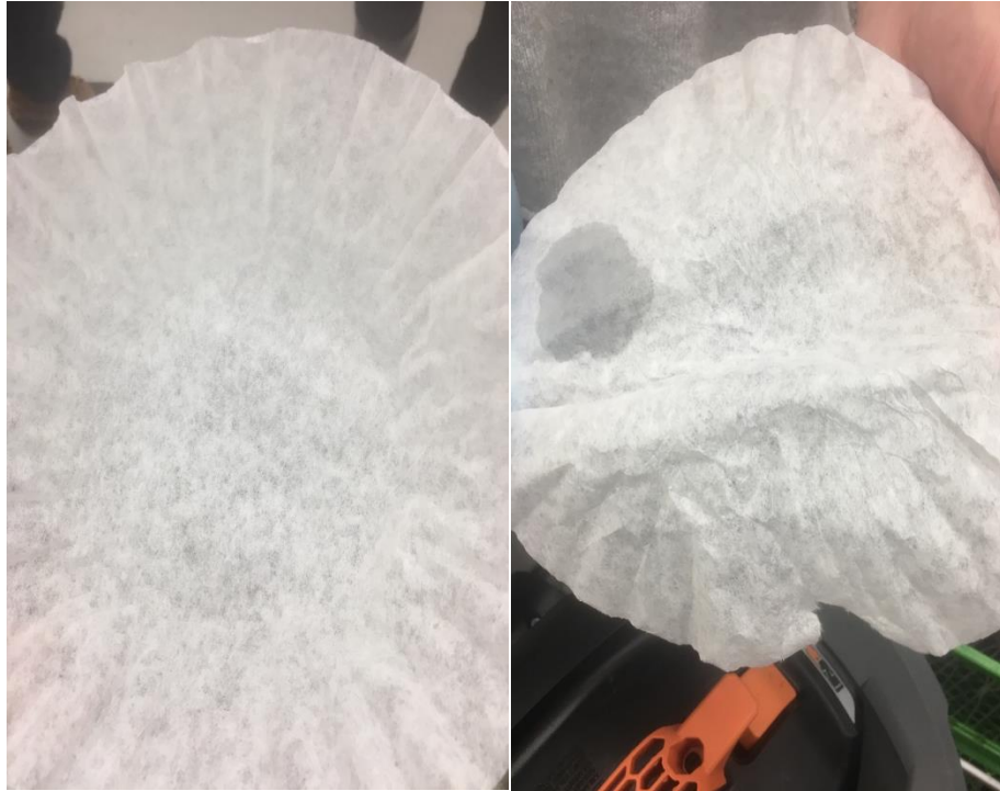
Figure E.1: coffee filter before running blue dye test (left), coffee filter after running blue dye test (right). Note: the small water spot on the filter pictured on the right was due to residual water on our hand, not water from the vacuum outlet.
