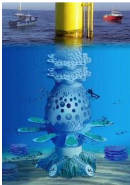
Figure 5: Example of design with increased surface area to promote the reef effect (Lacroix & Pioch, 2011).
